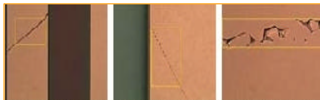
Figure 3. Copper scratch examples (detected using AIT II): a) razor scratch, b) chatter scratch, and c) skipping scratch.
